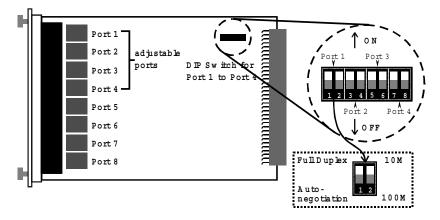
Figure 1-5. Dip switch location and mode settings
